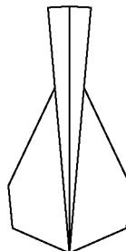
M9 9mm M882 Scale: 1:50,000 Distance X: 1,800m Impact Media: worst case Vertical Hazard: 253m
