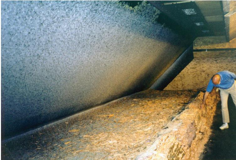
3.4.2 Escalator bullet stop (Figure 2). The escalator bullet stop has sloping steel surfaces to guide the bullet into a location where the projectile's energy can dissipate safely. The bullet travels up the surface of the plate to either a "swirl" area or deceleration chamber. Due to friction or multiple impacts, the bullet loses energy, then falls into a tray for later collection.
