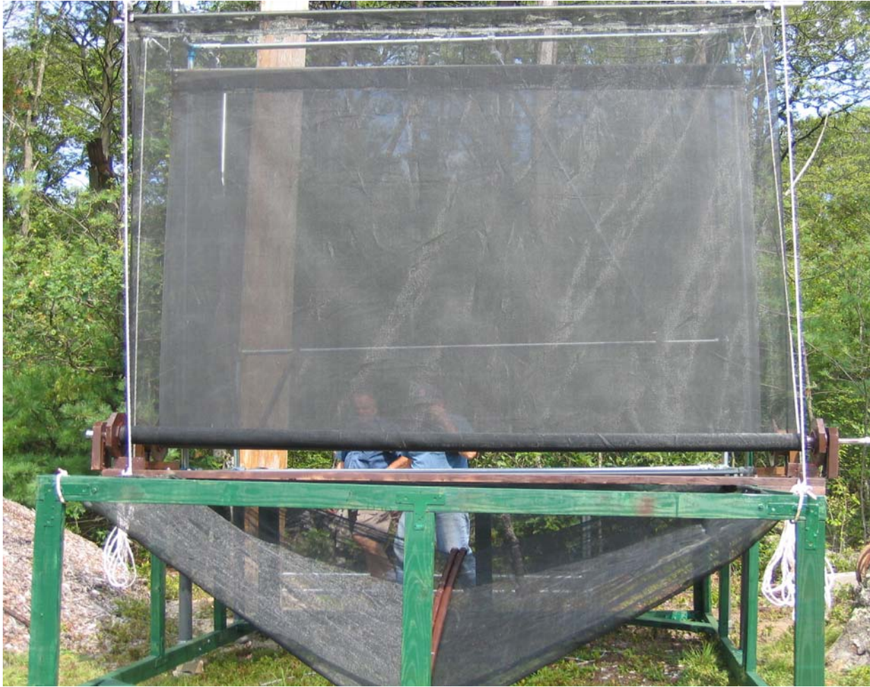
Figure 12: Photograph of Double Curtain Modular –Lead Pellet Capture System Located at the Standish Sportsmen’s Association Range.
