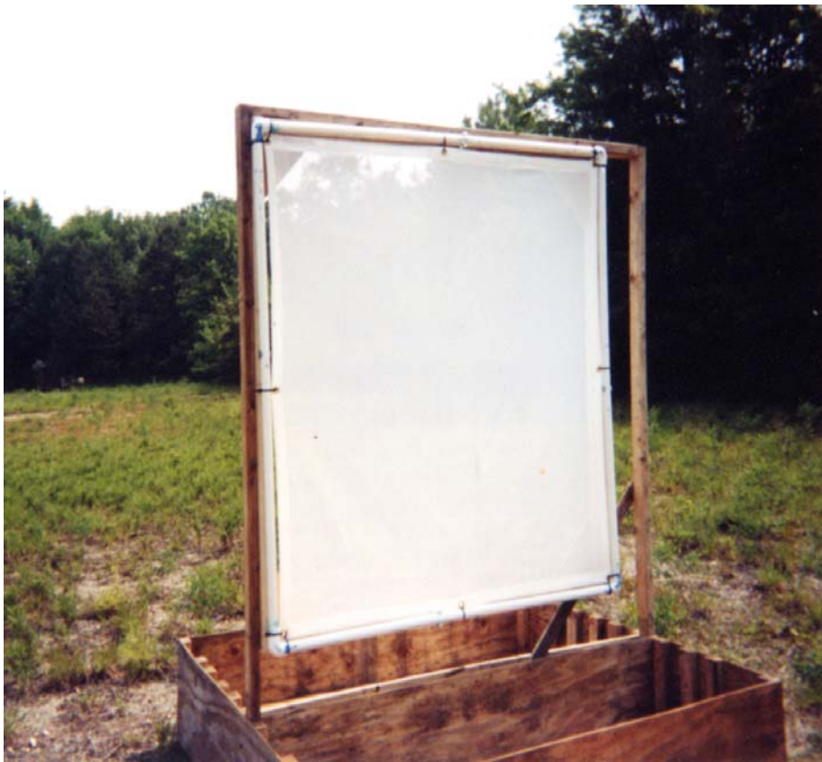
Figure 1: UMD In-Field Lead Pellet Impact and “Bounce-Back” Test for Evaluating Experimental LSC Fabrics. (A Framed 5 foot by 5 foot Fabric Test Panel is shown)
