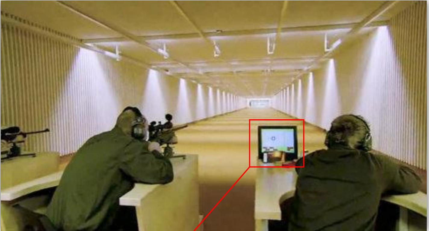
Although only shooting 25 meters (in reality), where there is no projectile drop, the target scoring software takes into account the image “distance” and compensates for how the projectile would have dropped at that distance and scores the shooter accordingly.
