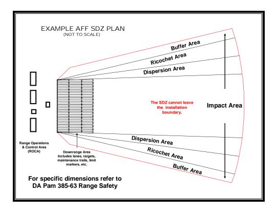
Definition per DA PAM 385-63: The ground and airspace designated within the training complex (to include associated safety areas) for vertical and lateral containment of projectiles, fragments, debris, and components resulting from the firing, launching, or detonation of weapon systems to include explosives and demolitions.
